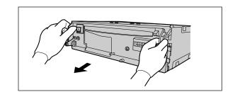
This unit is equipped with a removable face plate. Removing this face plate makes the radio totally inoperable. The security indicator will blink.
